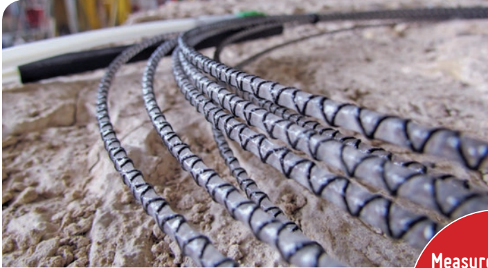
EpsilonSensor before installation in a lab specimen
