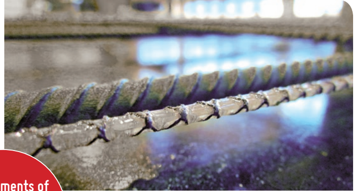
EpsilonSensor embedded into a reinforced concrete slab
